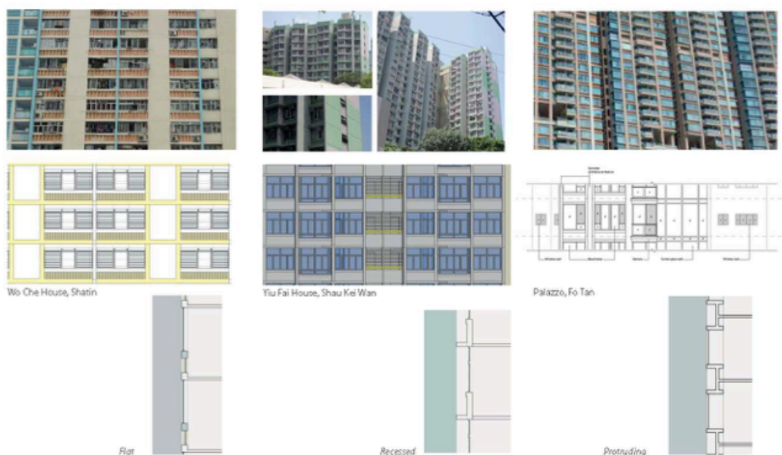
Figure 1 Three configurations of building envelope constructions that are representative of residential buildings in HK: flat, recessed and protruding.
