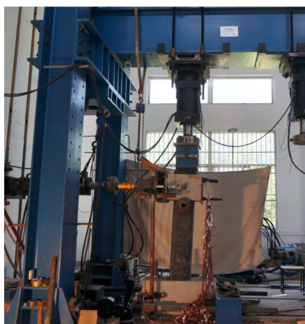
Figure 2(a) RC column tests - test setup and DIC system
