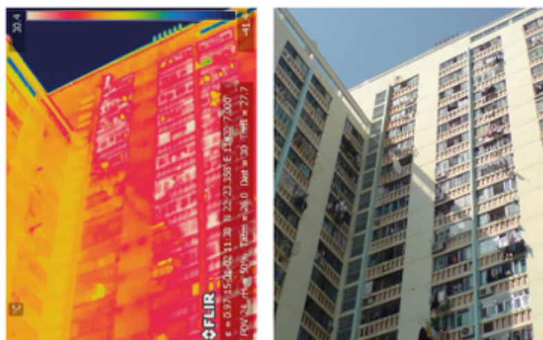
Figure 4 Thermal infrared image of a partially suncast building envelope. The radiant temperature difference at the envelope surface between suncast and shaded wall surfaces on same wall ranges up to 12.5 degree, about 61.6 W/m 2 radiant heat flux.
